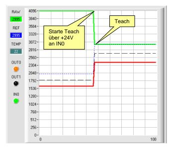
After a positive signal (+24V) at input IN0 the transmitter power is adjusted such that the sensor is in its dynamic range, which is set by **DYN WIN LO** and **DYN WIN HI**.
