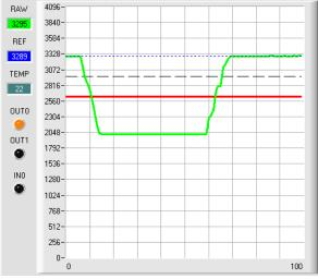
When the current measurement value **RAW** (green line) rises above the hysteresis threshold (black line) again, the output **OUT0** also changes to +24V again (signal is OK). This is visualised by the **OUT0** LED.
