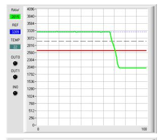
When the current measurement value **RAW** (green line) falls below the switching threshold (red line), the output **OUT0** changes to 0V (error). This is visualised by the **OUT0** LED.
